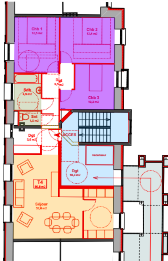
PLAN ETAGE TYPE Restructuration T4
