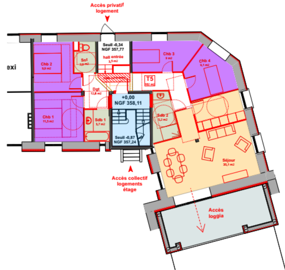
PLAN RDC Restructuration T5
