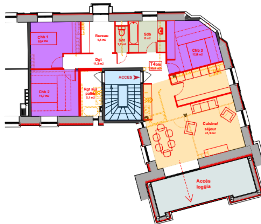
PLAN ETAGE TYPE Restructuration T4bis
